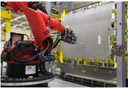
Automation of assembly for High Rate Production inc conventional and orbital drilling
