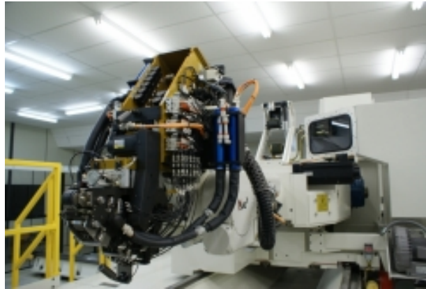
Bild 4 "Fiber Placement Machine" vid Lightweight Structures Laboratory i São José dos Campos.
