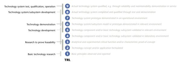
The degree of technological maturity (technology readiness level, TRL) is indicated using a nine-point scale developed by NASA and aims to highlight how far research on a particular technology has come before the innovation is fully developed into a manufactured, sold, and working product. TRL 0 indicates it is an idea, TRL 9 indicates it is a proven product on the market. Different research and development organisations are usually at different points on the scale. (Source: IFOT 12)
