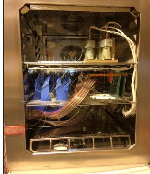
Temp. chamber, rigged with 8 test boards
